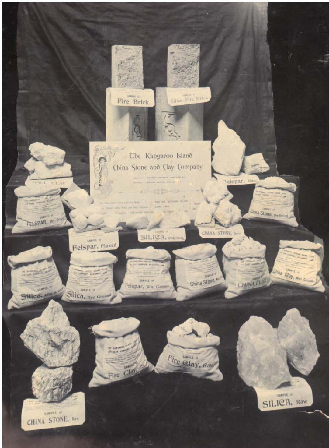
The Kangaroo Island China Stone and Clay Company trophy for the Franco-British Exhibition, London, was photographed at Penneshaw in 1908 before it was shipped. Samples included raw china stone, ground fire clay, raw and wet-ground silica, wet-ground feldspar, fluxed feldspar (used extensively for glazing ceramics), wet-ground china stone and, surmounted by split bricks, a fire brick and a silica fire brick stamped with the company logo (Penneshaw Maritime and Folk Museum).
