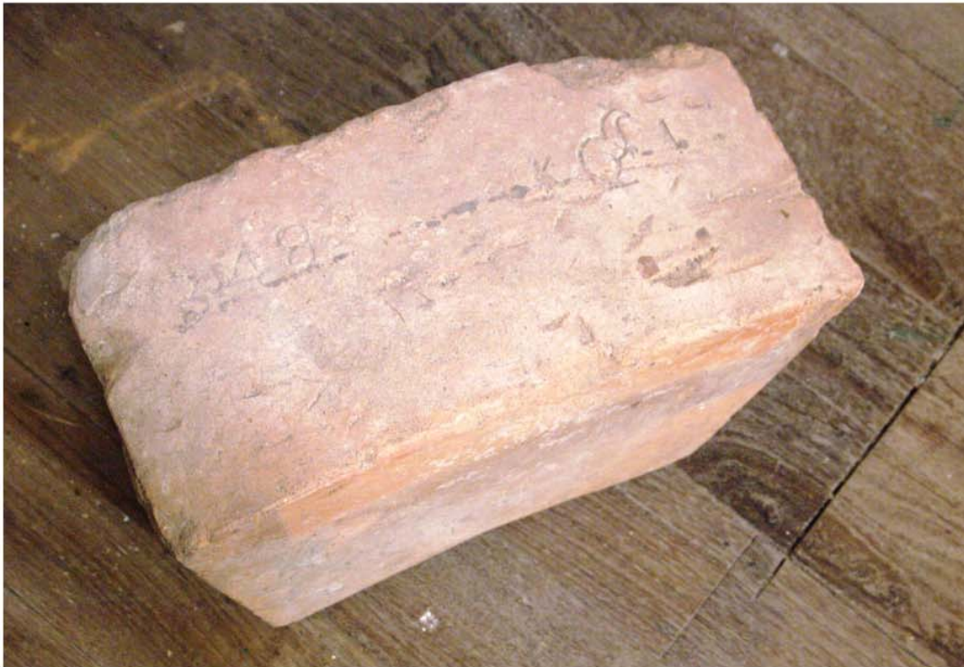
Tapered block, probably a voussoir, made at the Penneshaw brickworks (Penneshaw Folk and Maritime Museum)
